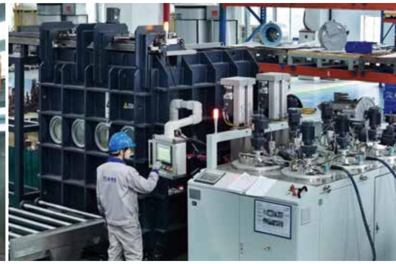
Epoxy resin vacuum pouring automatic line
