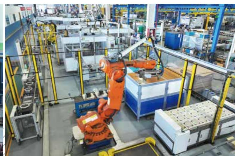
Robot shell hot sleeve assembly line
