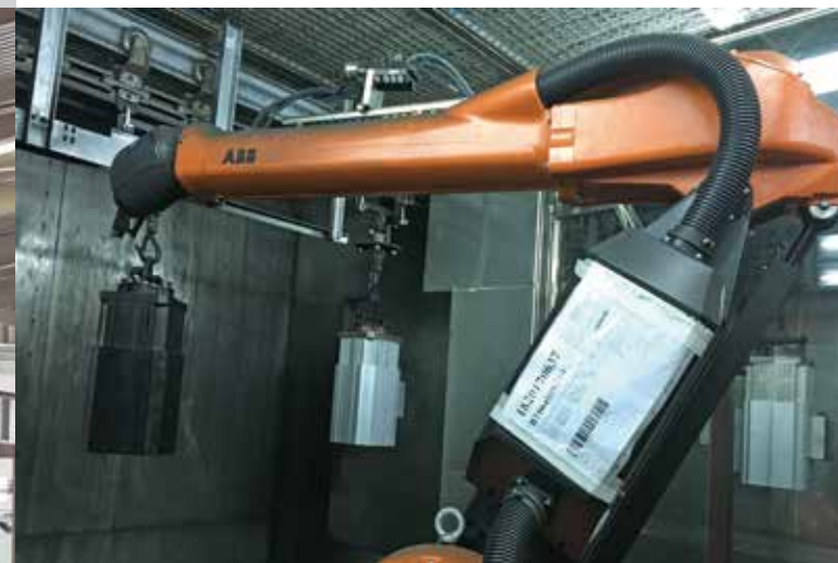
Robot Automatic Spray Painting Line
