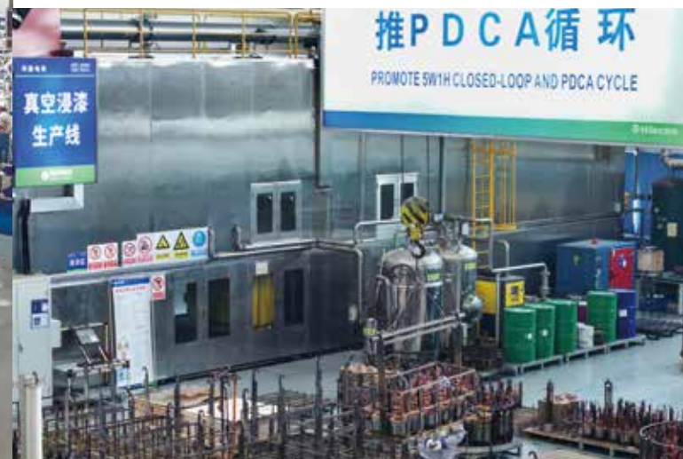
Vacuum Impregnation Line
