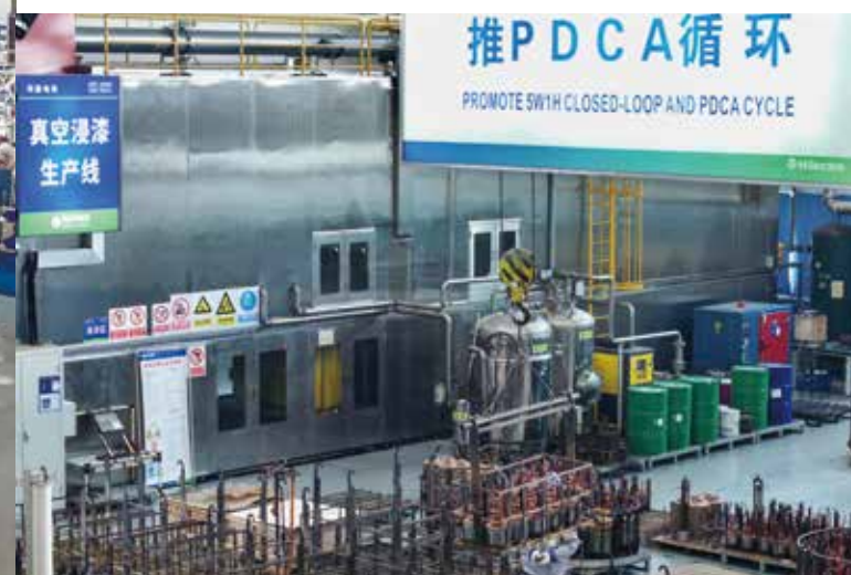
Vacuum Impregnation Line
