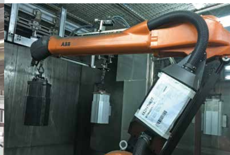
Robot Automatic Spray Painting Line
